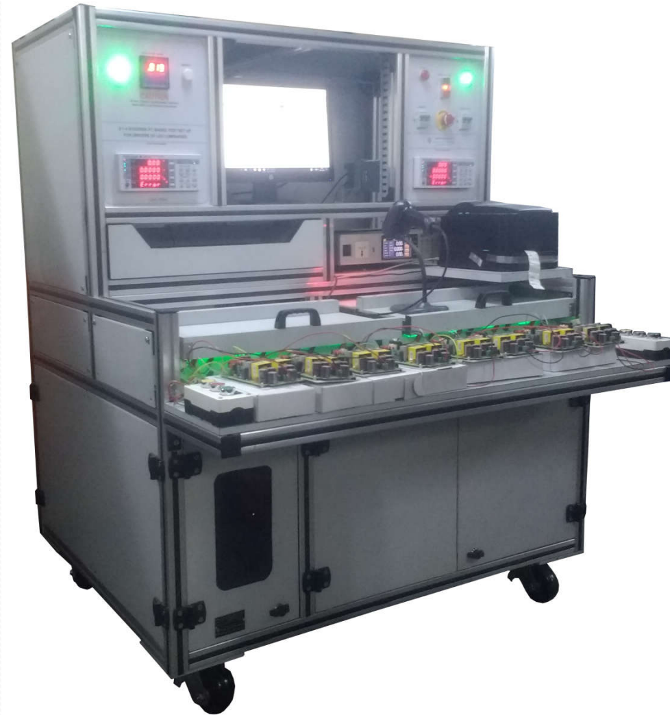
PC Based Test Set Up For 4 + 4 Drivers Of LED Lamps
