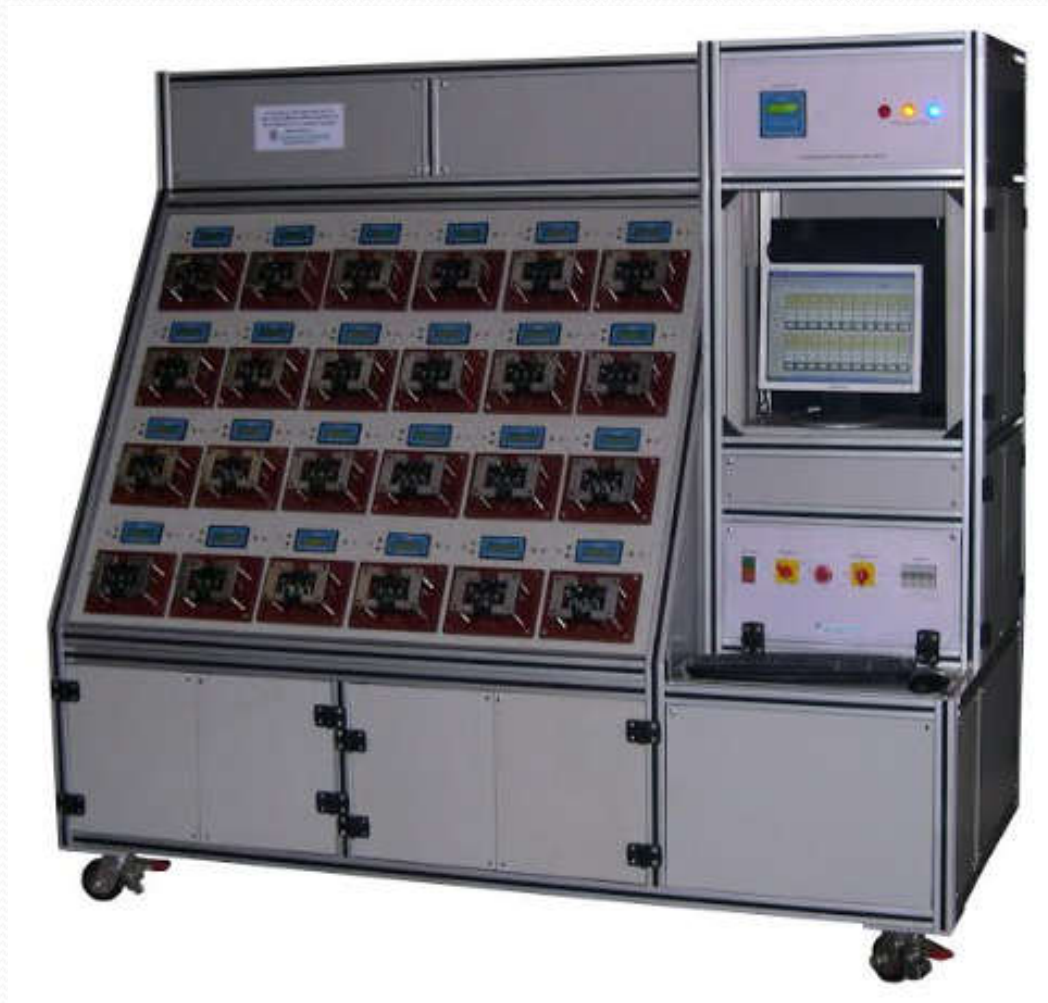
Relay Heating Routine Test Bench
