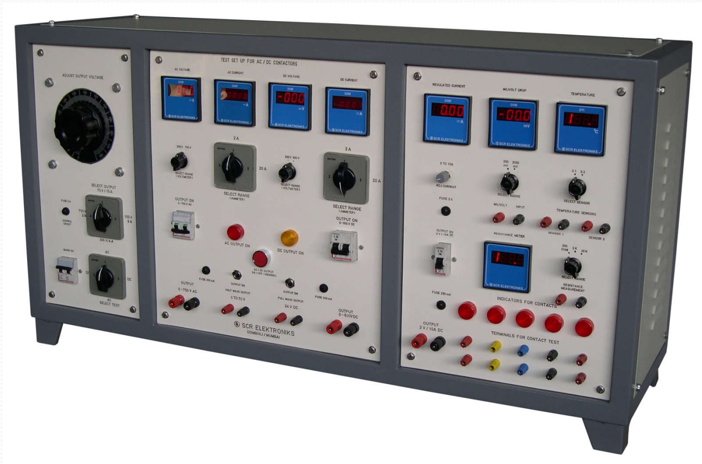
Contactor Prototype R&D Test Bench
