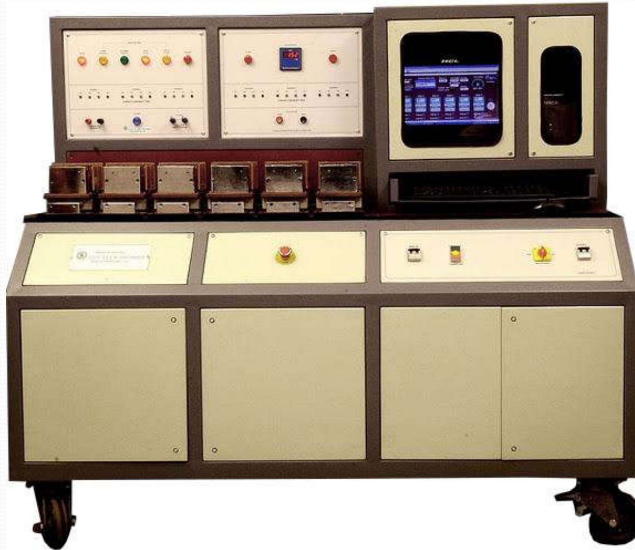
Routine Test For Contactors
