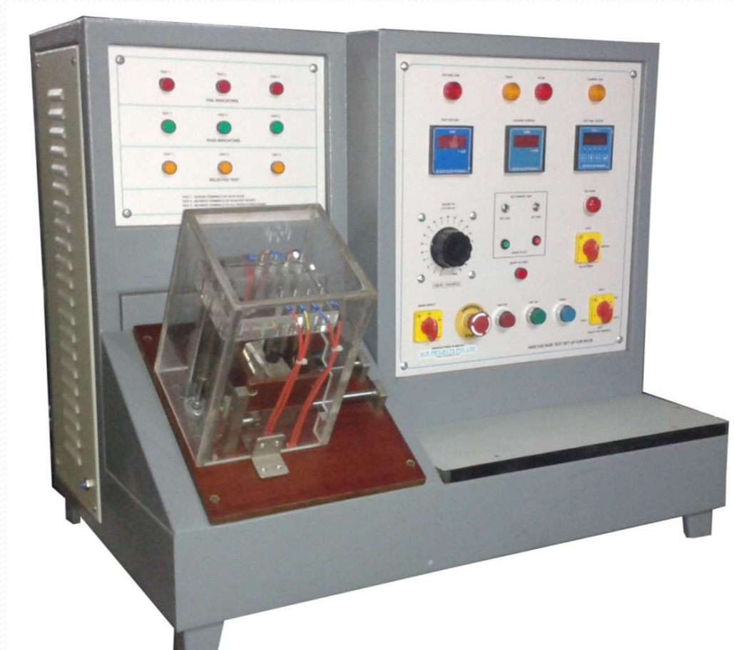
High Voltage Test Setup For RCCB
