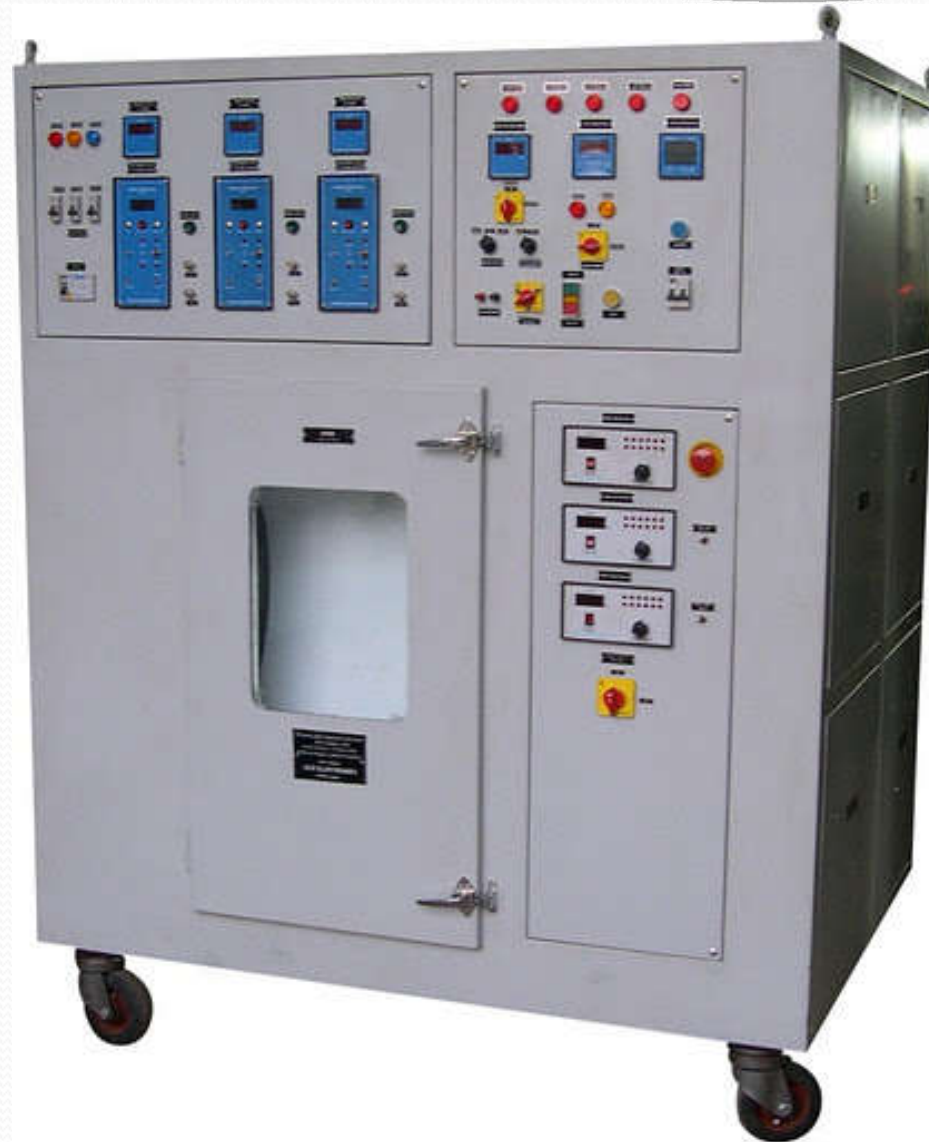
28 Days & Temperature Rise Test Panel For RCCB/RCBO
