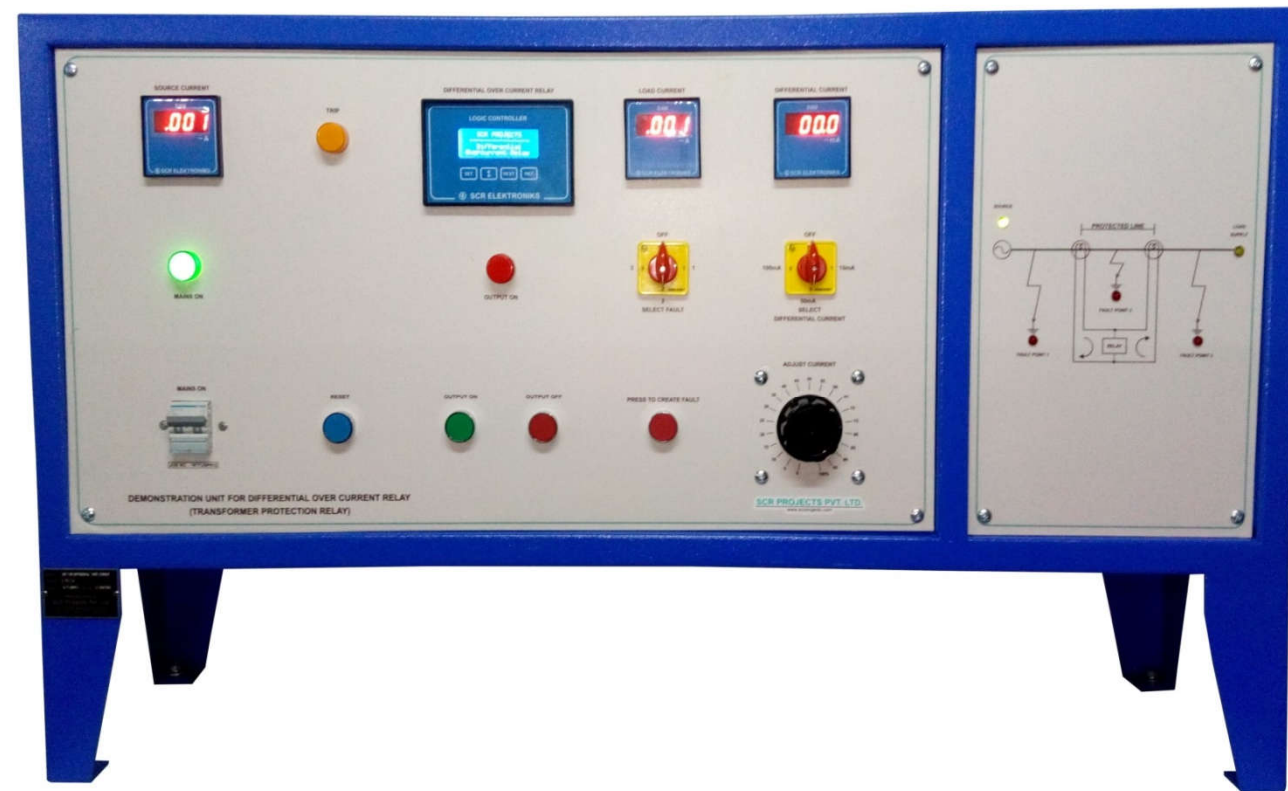
Demonstration Unit For Differential Over Current Relay
