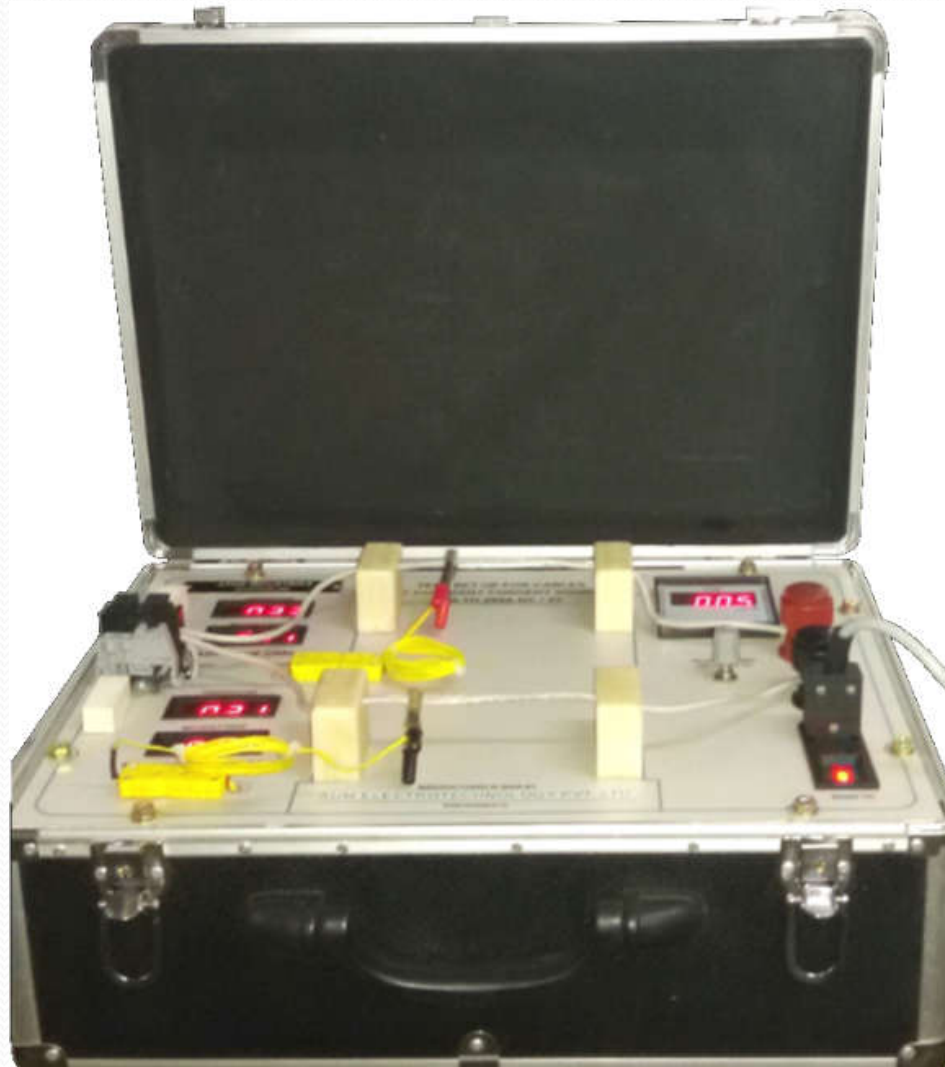
TEST SETUP FOR FLEXIBLE PERFORMANCE OF WIRES & CABLES
